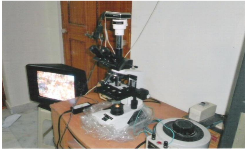
Polarizing optical microscope (SDTECHS make) The textural and phase transition temperatures
