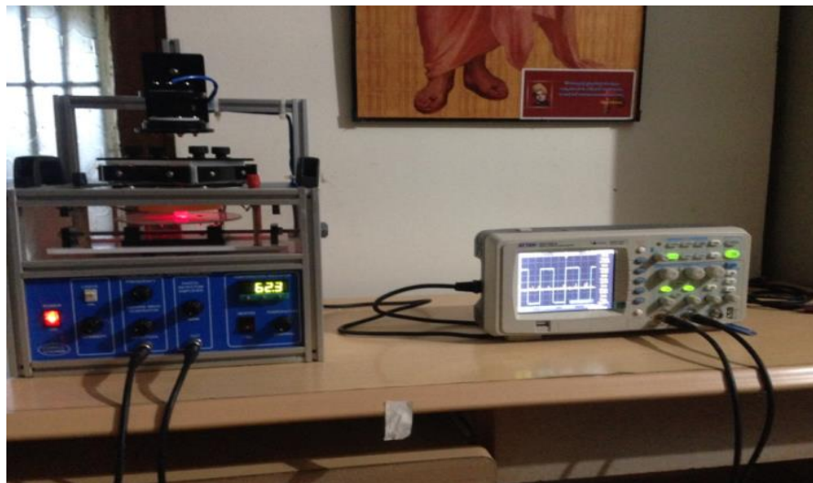
Indigenously designed and fabricated Digital Birefringence Spectrometer
