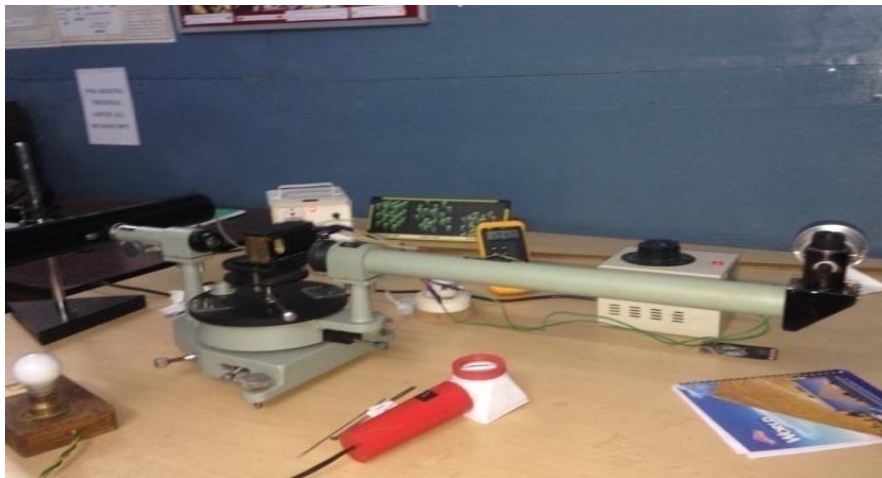
Modified Spectrometer – Determination of refractive indices ( n_e & n_o ) of Liquid Crystals
